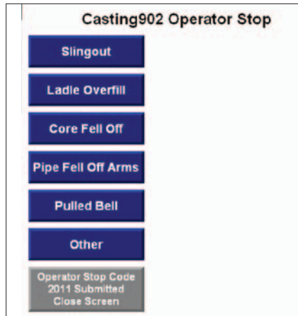
Figure 2. HMI screens allow operators to choose from several categories of operator stops. Once operators select the downtime category, they can then select a more detailed reason for the downtime.
