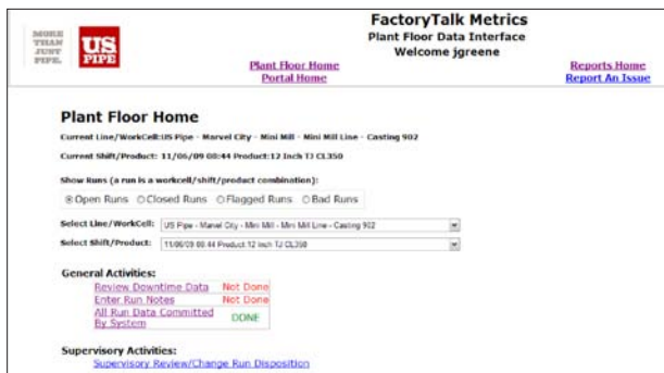
Figure 3. This screen allows the operations team to clarify data that the system recorded. The operations engineer selects the operation for which he/she wants to modify data, the shift and product. The user then can review downtime events and make any necessary modifications, such as splitting events into multiple time buckets, changing descriptions or adding notes.
